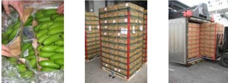
Fig. 2. (a) Placement of Wireless Sensor Network node in the food box (b) Packed pallet (c) Loaded cargo container
