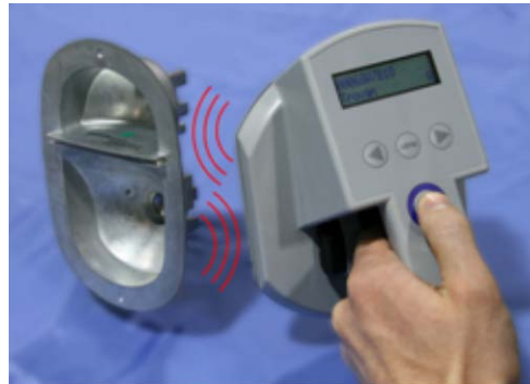
Figure 7: Die-cast rear light with embedded RFID
