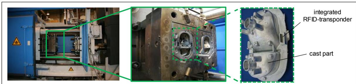
Fig. 5: Die-cast unit FRECH DAW 315 (left), die casting mold (center) and final cast part with integrated RFID transponder (right)
