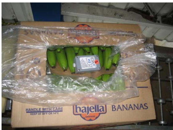
Fig 6: Wireless sensor nodes (left) and data logger in two additional boxes (right)
