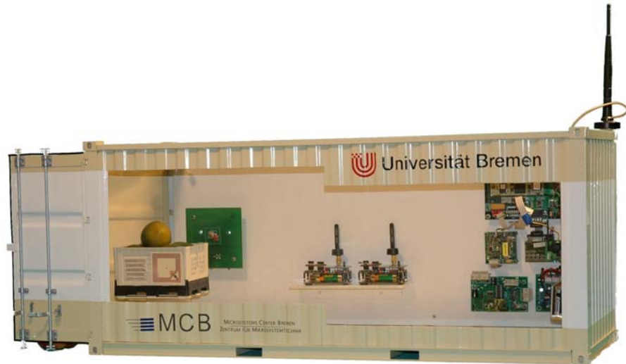
Figure 4: Reduced scale (1:8) prototype of the intelligent container. Loaded freight items are scanned by the RFID-Reader on the left. Sensor nodes supervise the environmental conditions 7 (middle). A processor module on the right side executes a software agent containing specific transport instructions and quality modelling. The module for external mobile communication is placed on the right side panel.
