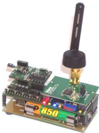
Fig. 3: Sensor node for wireless transmission of measurement values inside the means of transport. Modules for temperature, humidity, light and vibrations are available.
