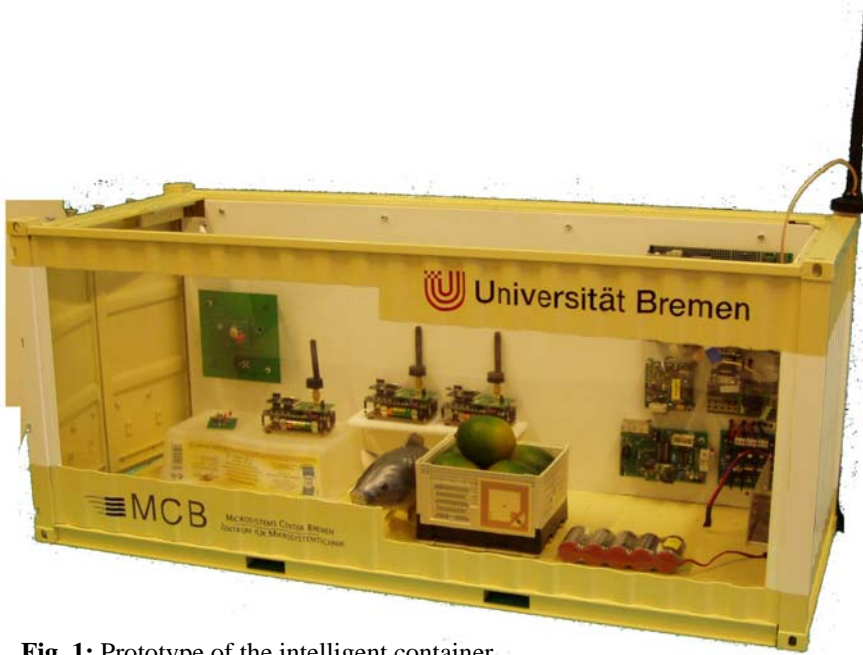
Fig. 1: Prototype of the intelligent container. Loaded freight items are scanned by the RFID-Reader on the left. Sensor nodes supervise the environmental conditions (middle). A credit card sized processor module on the right side executes a software agent containing specific transport instructions and quality modelling. The module for external mobile communication is placed on the right side panel.
