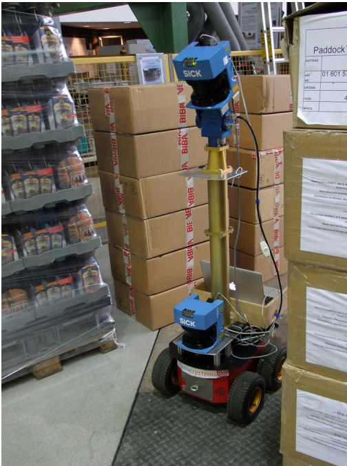
Figure 1: A Pioneer-3 mobile robot platform equipped with a 3D laser range unit in an experimental storage environment. RFID readers are not mounted to the platform in this picture.
